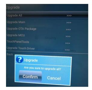
4. The power LED will keep twinkle in red and blue during upgrade process. After finished, the panel will reboot and enter Android channel. It will take 3 minutes to complete the upgrade procedure.
