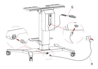
Step2: Plugging the AC Power transferable Cable and the USB transferable Cable in, user can interact with the Interactive Flat Panel.
