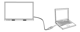
Turn on the IFP, connect the EasiCable to the side USB port of IFP with the standard USB touch cable.
